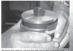
Re-form the seal by squeezing the wear ring over the seal.
