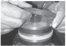
Place a nylon wear ring - 1/4" larger diameter than the piston -
