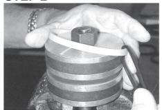
With your hand over the edge of the piston and holding the seal with your palm, cut and loop an o-ring through the seal. With one motion, pull down and around until the seal is on the piston. Now, remove the o-ring.
