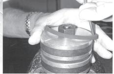
Lubricate and install the rubber expander ring into the groove as shown.
